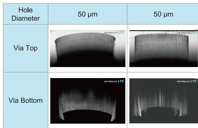
Capturing TSV Striation Cross-Section and 3D Imaging
